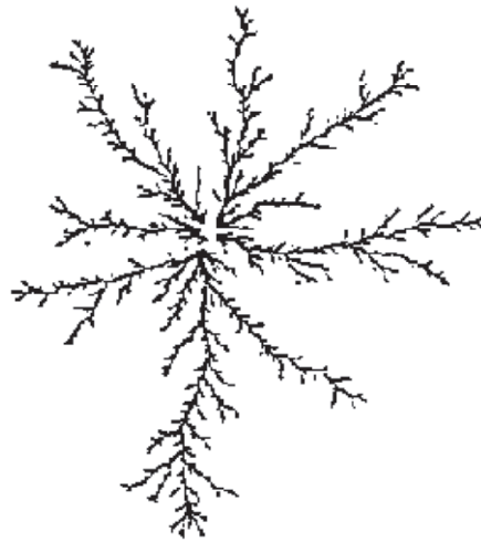
Fig. 2.20. Growth of a dendrite. The Zn dendrite grows according to a fractal structure. It is obtained by electrodeposition of metallic Zn at the interface between an aqueous solution of Zn sulfate and n -butyl acetate (M. Matsushita et al., Phys. Rev. Lett., 53 , 286 (1984), copyright Am. Inst. Phys.)
