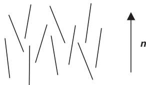
Fig. 8.2. Nematic phase. In each monodomain, the molecules are oriented in a preferred direction \mathbf{n} , but the positional order of the molecules is close to the order in a normal liquid
